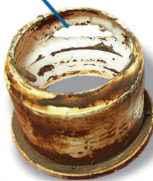
WORN, FAILED BEARING
