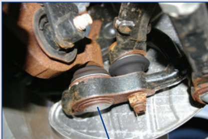
OE BALL JOINT (NON-SERVICEABLE)
