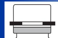
Welded plate bearings: remove grease boots and ensure caps are fully seated by applying light pressure using a C-clamp or a vise at both ends of cups (tight enough that the u-joint cross body can be turned by hand). Measure the distance between the opposite plates. Don't include the plate thickness in the measurement.
