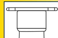
Winged bearings: measure the distance between the holes directly across from each other and the pilot diameter. Make sure to take note of the style of the wing as there are many variations.
