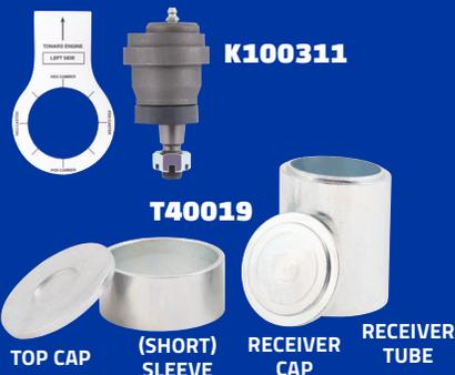
The MOOG ball joint press tool T40019 makes installation of MOOG adjustable offset ball joints easy. The sleeve in the T40019 is designed to match the angle of the yoke on the axle housing to ensure proper installation. Use in conjunction with the T40001 C-clamp ball joint press.
